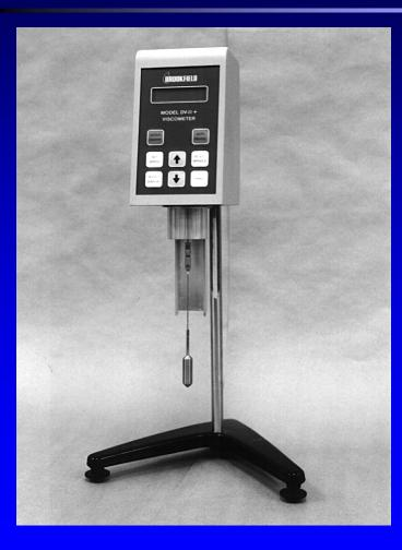
Rotational Viscometer (Brookfield) ► Measures viscosity at 135°C and 165°C ► Viscosity @ 135°C < 3.0 Pascal seconds Determines Equi-viscous Lab Mixing and Compaction Temperatures Does not work for PMA - use suppliers recommendations **Does not determine field** *temperatures*
