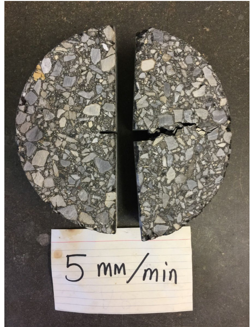
Specimens Before (L) / After (R) Testing
