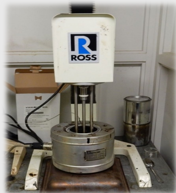
Blending equipment with heating mantle
