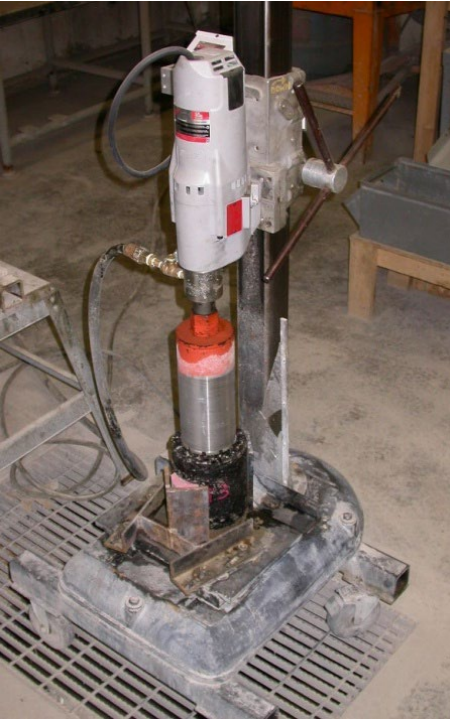
Coring (left) and sawing (right) of a gyratory compacted specimen
