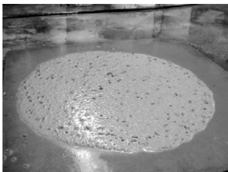
VSI = 2; Mortar halo, slight segregation
