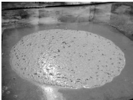
VSI = 2; Mortar halo, slight segregation
