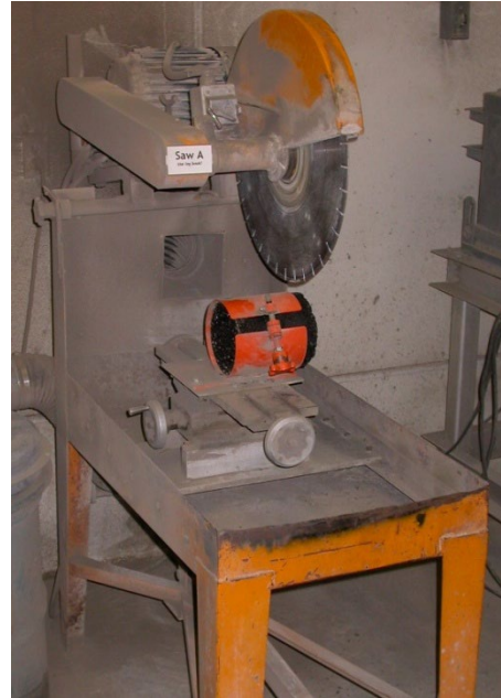
Coring (left) and sawing (right) of a gyratory compacted specimen
