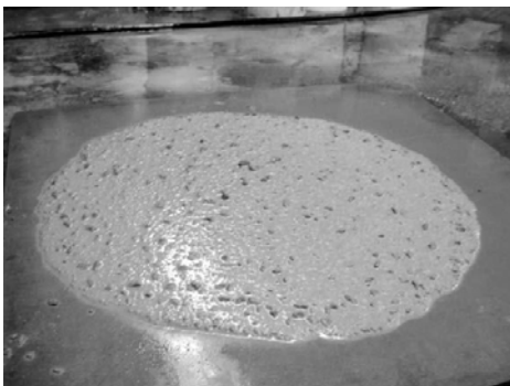
VSI = 2; Mortar halo, slight segregation
