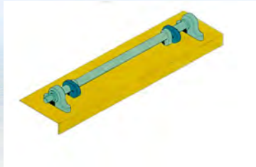
Vibratory Shaft with Weights
