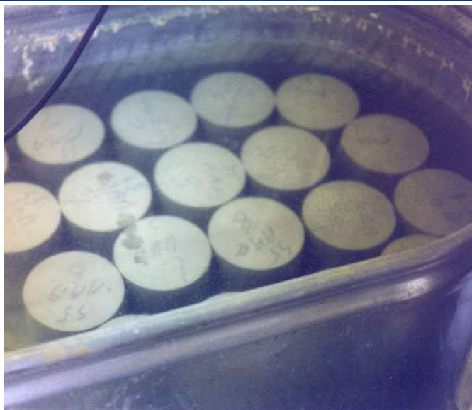
AT & VT cylinders Saturation in lime water tank
